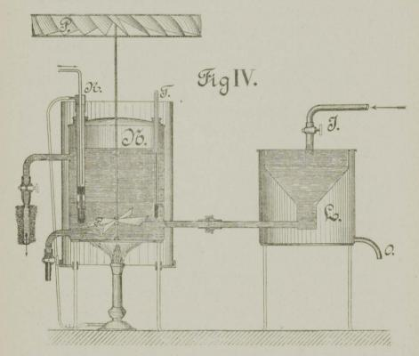
fluous water flows into the vessel placed round L, and streams of through O.
