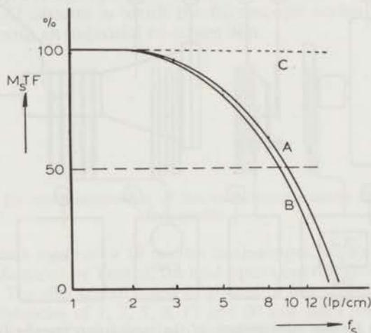
Fig. 12. Comparison of two photographic methods for the determination of the  $M_s TF$ . Curve A obtained by contact printing, curve B obtained with the camera, dotted curve C Leica camera with Leitz lens.
