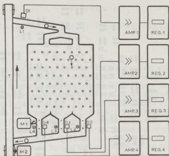
Fig. 17. Diagram of the apparatus for measurement of image quality.
