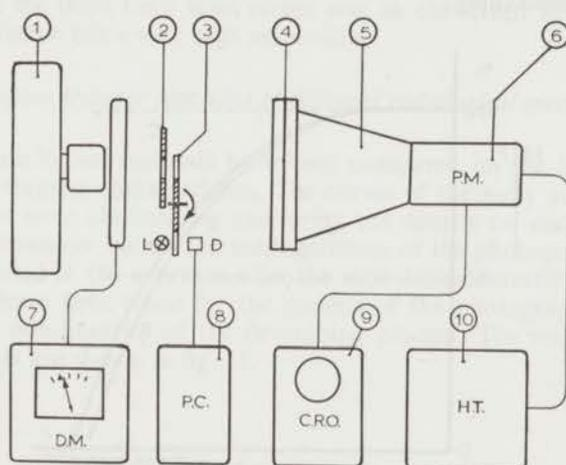
Fig. 11. Diagram for the measurement of the modulation transfer function of time frequencies.
