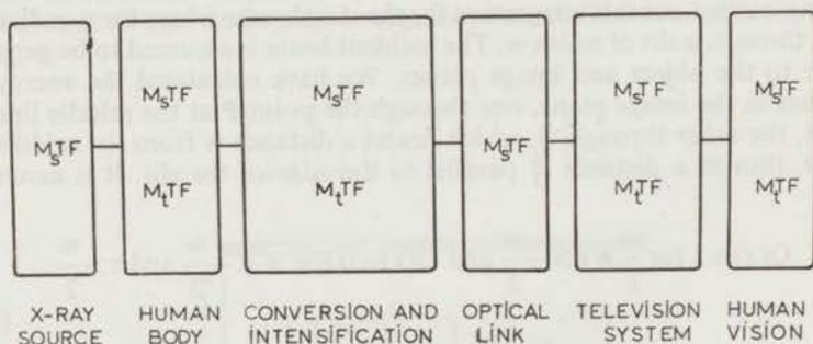
Fig. 3. Image deterioration in fluoroscopy.
