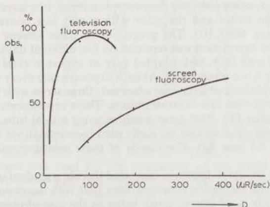
Fig. 20. Comparison of direct screen and television fluoroscopy.
