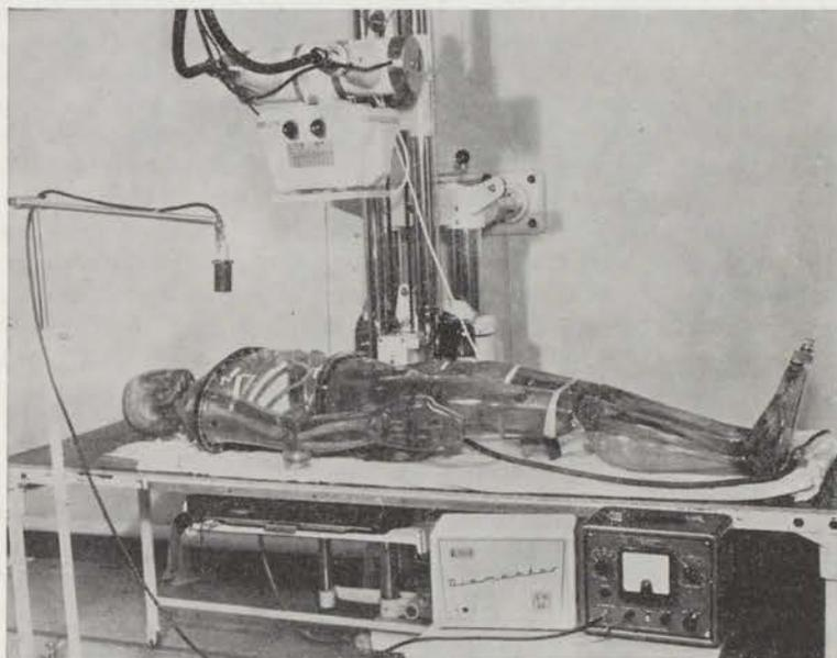
Fig. 21. Phantom used for radiation measurements.
